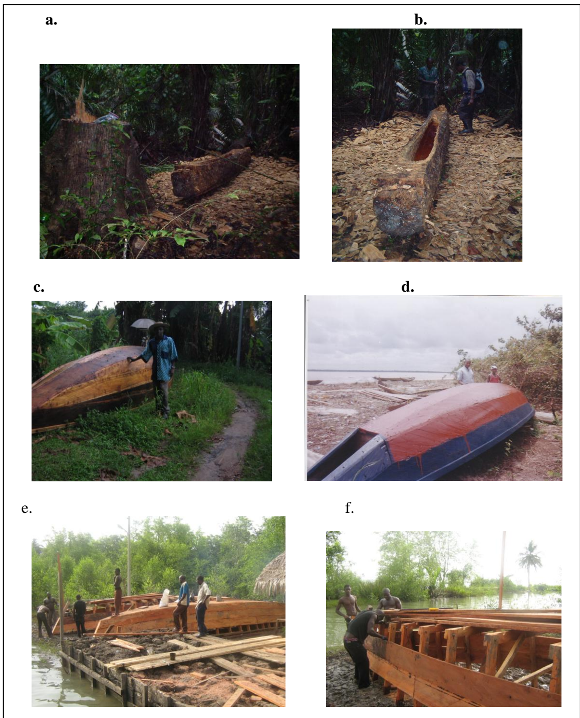
Plate 4.5: Canoe carving and boat building in the study area (a) Stump of tree felled for canoe carving in Oginibiri forest, (b) Initial stage of canoe carving shown, (c) Researcher standing by a boat under construction in Sangana community, (d) Wooden boat carved and painted in Opu-Okumbiri community, (e) Two wooden boats under construction on the mudflats along Ereweibie creek and (f) Side view of a wooden boat
