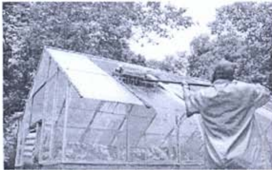
Fig 9. Greenhouse Roof Cleaning using the Designed Cleaner
