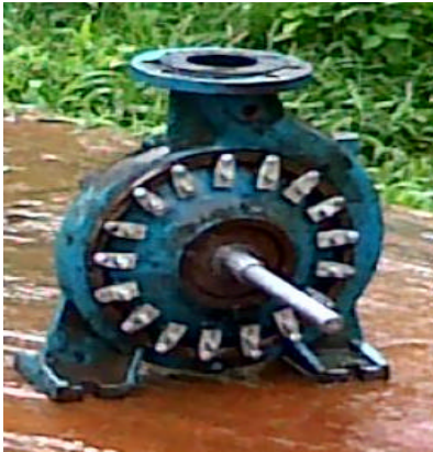
Fig. 16: Back view of turbine assembly
