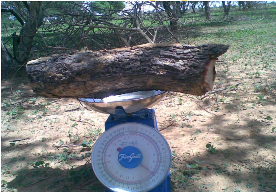
Plate 3.4: Determination of the fresh weight of the stem of Acacia senegal tree using weighing balance.
