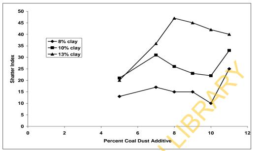
*Figure 3:* Plots of Shatter Index variations with coal dust additives for sand mixtures containing 8%, 10% and 13% clay, with 5% moisture content respectively
