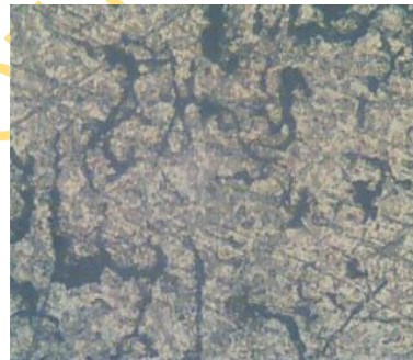
(b) 0.5% Cr, annealed at 800°C
