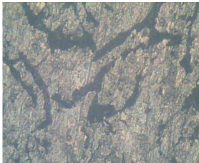
(a) Unalloyed, annealed at 800°C
