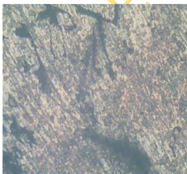
(c) 1.5% Cr, annealed at 800°C
