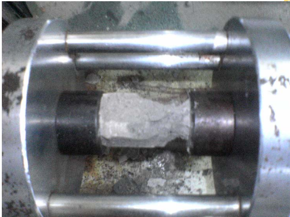
Fig.4: Brick fracturing during compression
