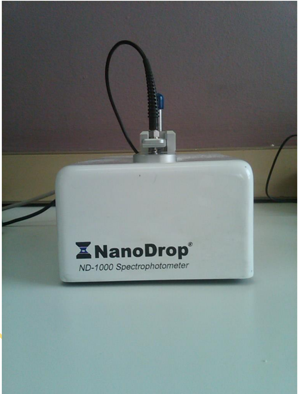
Plate 10: ND- 1000 Spectrophotometer used for DNA Quantification
