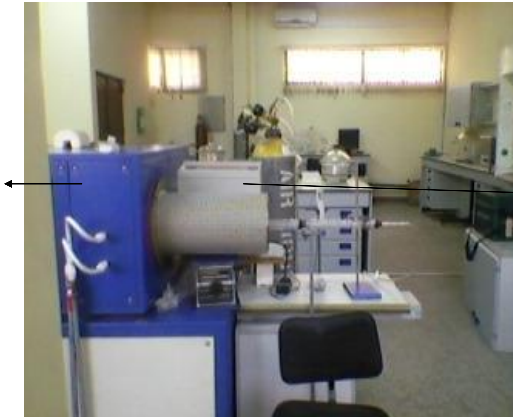
Fig.3.12. Sulphur vaporization section of the annealing process at the Physics Advanced Laboratory of the Sheda Science and Technology Complex, Abuja
