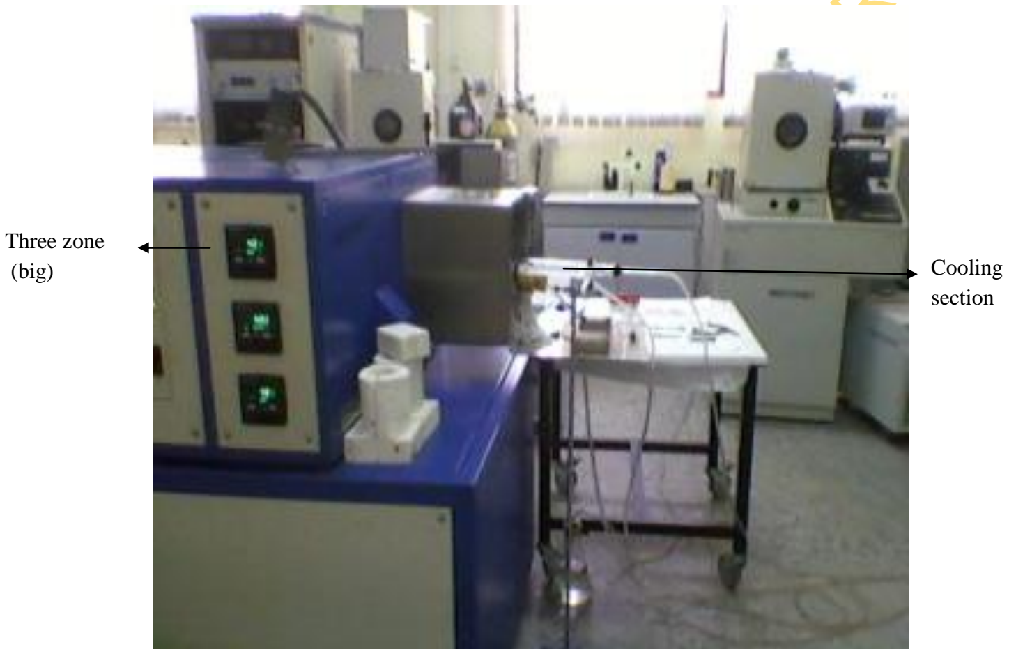
Fig.3.13. Cooling section of the furnace during the annealing process at the Physics Advanced Laboratory of the Sheda Science and Technology Complex, Abuja
