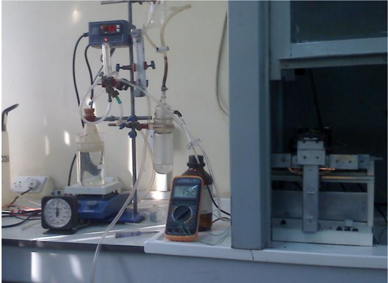
Fig.3.3. The entire APCVD set-up showing the arrangement of the precursor, dopant and depositing section.
