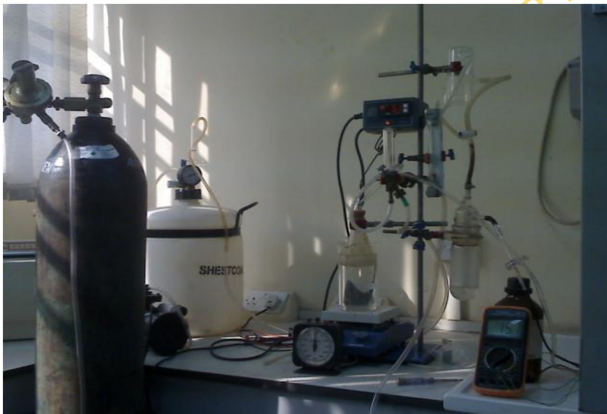
Fig.3.2. Precursor section of the APCVD set up at the Sheda Science and Technology Complex
