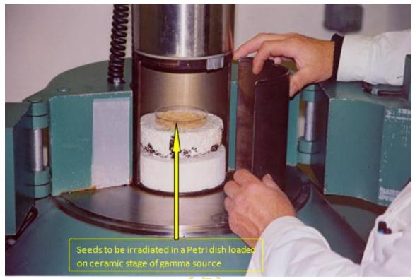
**Plate** 3.1. Close-up of the raised loading stage of Cobalt-60 gamma source showing seeds to be irradiated at IAEA
