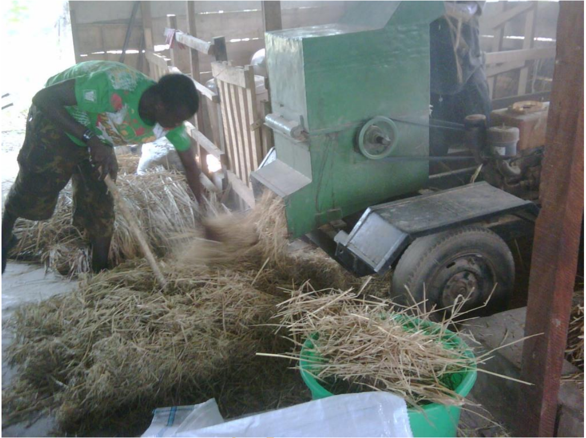
Plate 5: Chaffing of dried rice straw in a locally made chaffing machine
