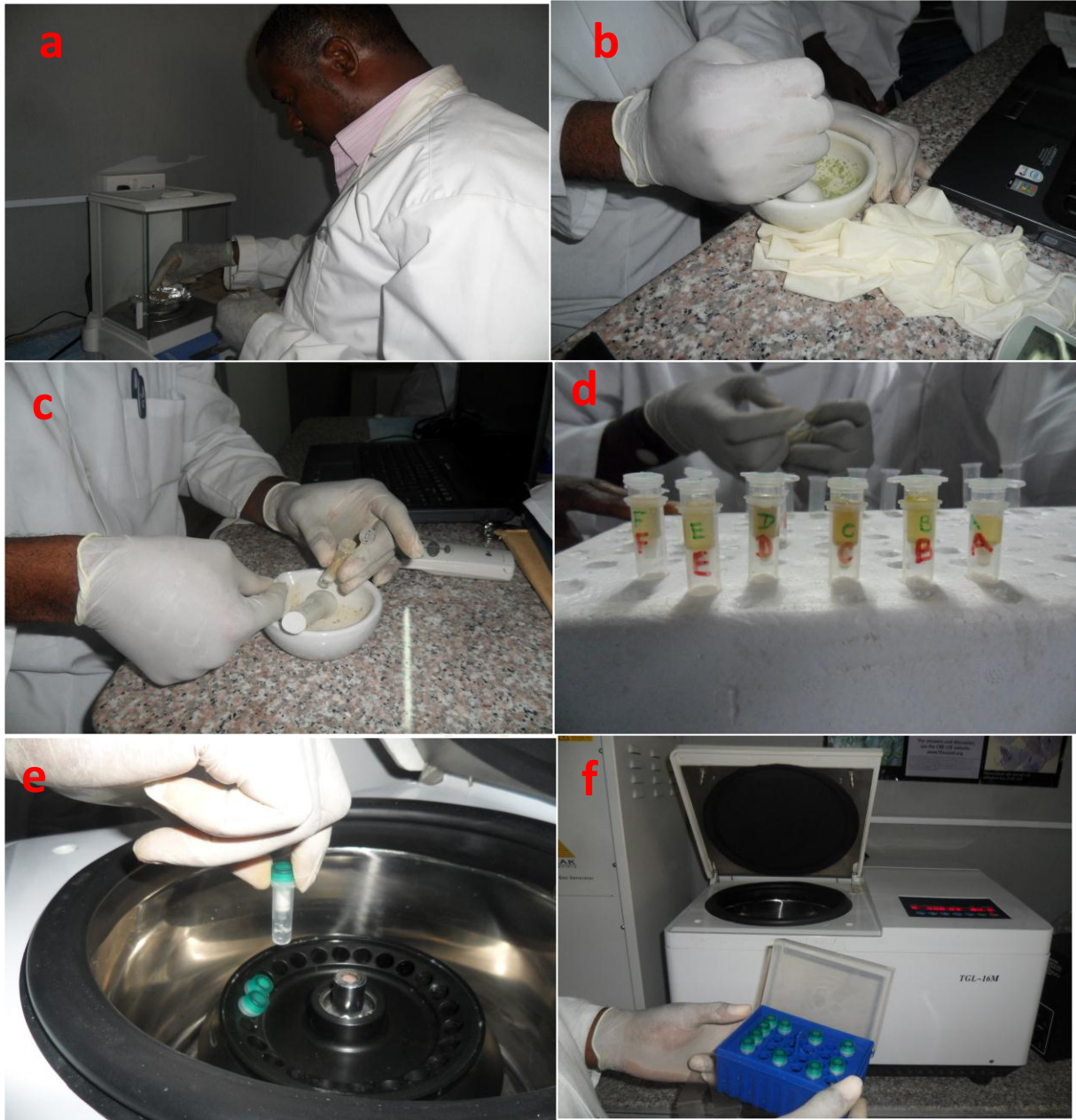
Plate 3.7: DNA extraction and purification process (a) weighing of sample, (b) grinding of sample, (c) collection of the ground sample into Eppendorf tube, (d) well labelled collected samples (e) samples arranged in the centrifuge and (f) centrifuged samples.
