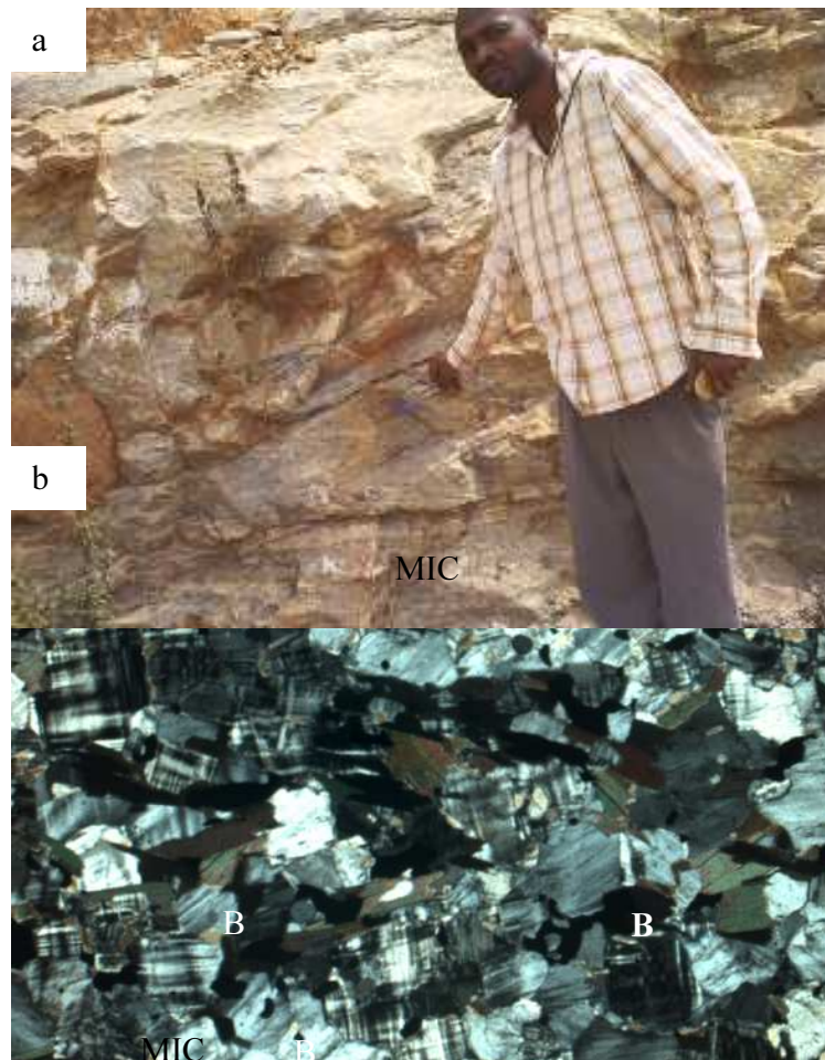
Figure 4.12: (a) Granite gneiss samples (b) Photomicrograph (crossed nicol) of one the samples. H= hornblende, B= Biotite, Qtz= Quartz, Plg= Plagioclase, M= Muscovite
