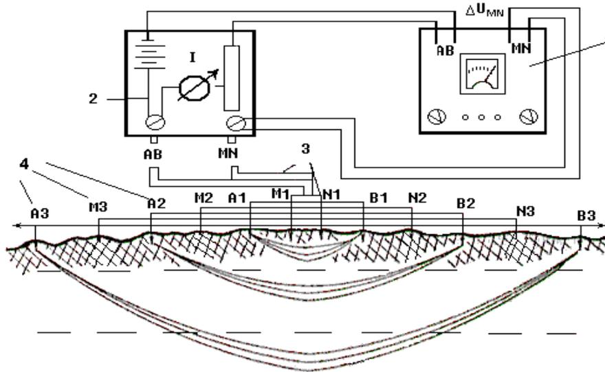
Figure 2.2: Scheme of the Vertical Electrical Sounding (VES) device: (1) auto-canceller, (2) commutator for electrodes AB and MN, (3) netted wires for different distances among electrodes AB and MN, and (4) electrodes ([http://larisa\\_pozd.tripod.com/ves/ves.htm](http://larisa_pozd.tripod.com/ves/ves.htm))
