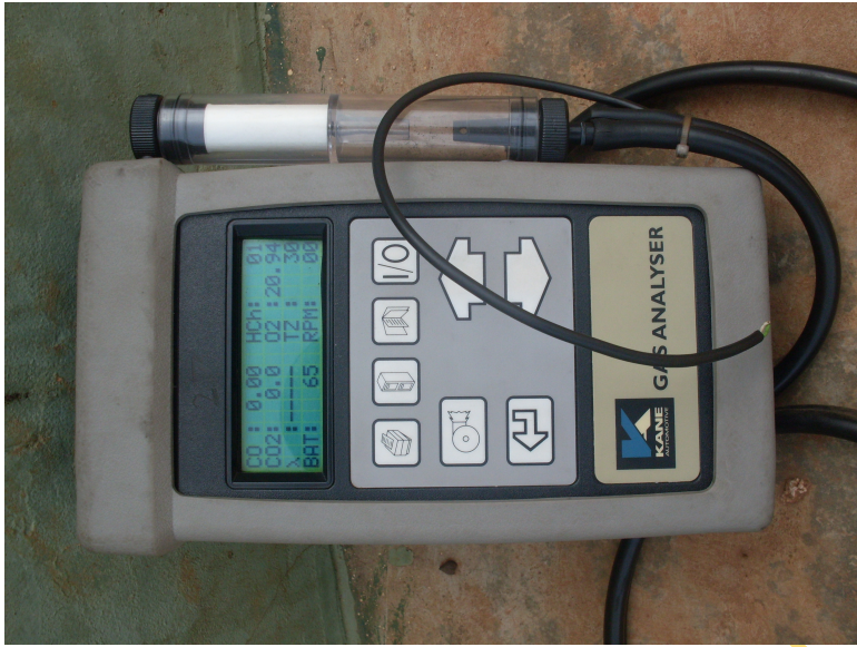
Figure 5.7: Kane Gas Analyser
