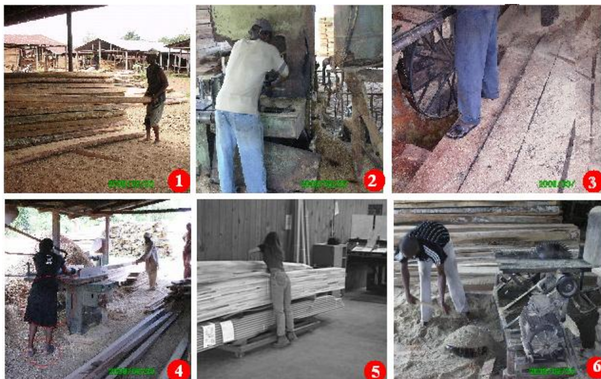
Figure 1: Identifiable hazards in sawmill sites: 1) Manual Lifting and stacking sawn lumber, 2& 3) Non-use of protective wears and equipment during maintenance, 4 & 5) Repetitive motion, twisting and reaching for objects and 6) Breathing in of noxious or toxic chemical emissions during waste disposal with head pan
