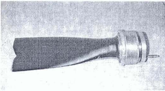
Fig.5: Broken propeller of the airplane [2].
