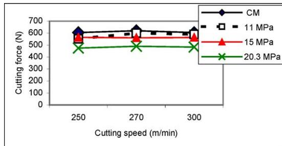
Fig. 4. Cutting forces recorded when finish machining with whisker reinforced alumina ceramic cutting tools at various cutting speeds and a feed rate of  $0.2 \text{ mm rev}^{-1}$ .
