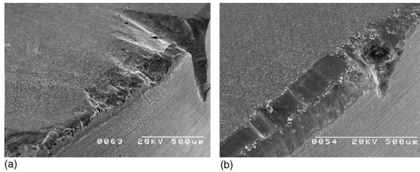
Fig. 3. Flank and notch wear after machining Inconel 718 (a) with 20.3 MPa coolant supply at a speed of  $300 \text{ m min}^{-1}$  a feed rate of  $0.2 \text{ mm rev}^{-1}$  and (b) with conventional coolant at a speed of  $270 \text{ m min}^{-1}$  a feed rate  $0.2 \text{ mm rev}^{-1}$ .
