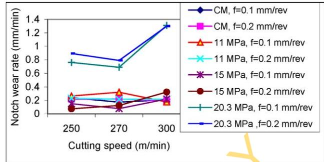
Fig. 2. Notch wear rates at various speed conditions when finish machining with whisker reinforced alumina ceramic tools.
