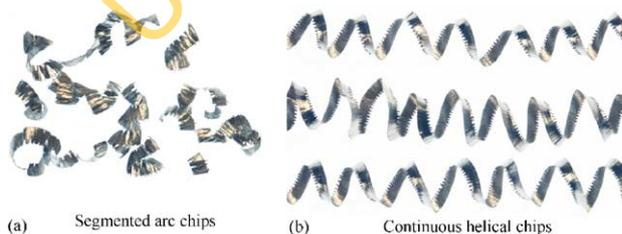
Fig. 5. Chips generated when finish machining Inconel 718 with whisker reinforced ceramic tools under (a) coolant supplies up to 20.3 MPa (b) conventional coolant flow.
