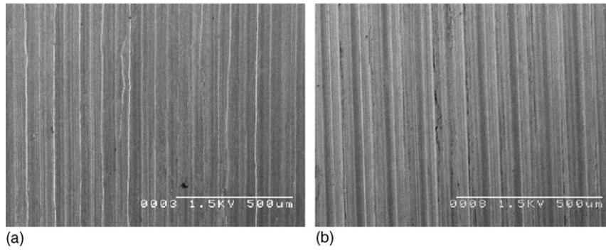
Fig. 7. Surfaces generated after finish machining Inconel 718 with whisker reinforced  $\text{Al}_2\text{O}_3$  ceramic tools with 15 MPa coolant supply (a) at a speed of  $250 \text{ m min}^{-1}$  and a feed of  $0.1 \text{ mm rev}^{-1}$  and (b) at a speed of  $270 \text{ m min}^{-1}$  and a feed of  $0.1 \text{ mm rev}^{-1}$ .
