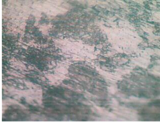
Fig. 7: Microstructure of annealed NST 37-2 steel (x400)
