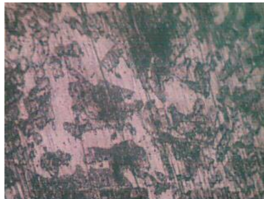
Fig. 6: Microstructure of untreated NST 37-2 steel (x400)
