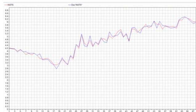
Fig. 3: Comparison between the ANN predicted and actual solar radiation for the month of January in Africa
