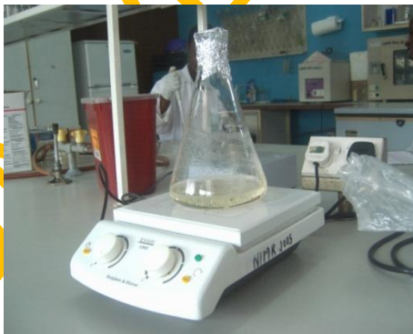
Boiling an Agarose gel on electrothermal plate
