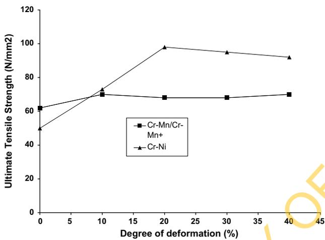
Fig. 4b. Variation of ultimate tensile strength with degree of deformation at 350 °C.
