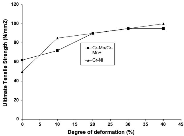
Fig. 4a. Variation of ultimate tensile strength with degree of deformation at 28 °C.
