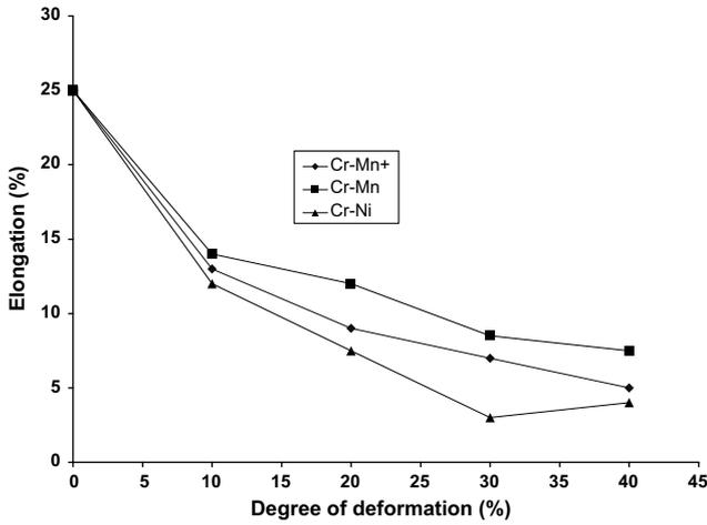
Fig. 2a. Variation of elongation with degree of deformation at 28 °C.
