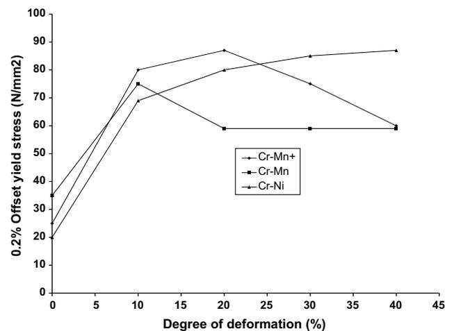
**Fig. 1c.** Variation of 0.2% offset yield strength with percent deformation at 650 °C.
