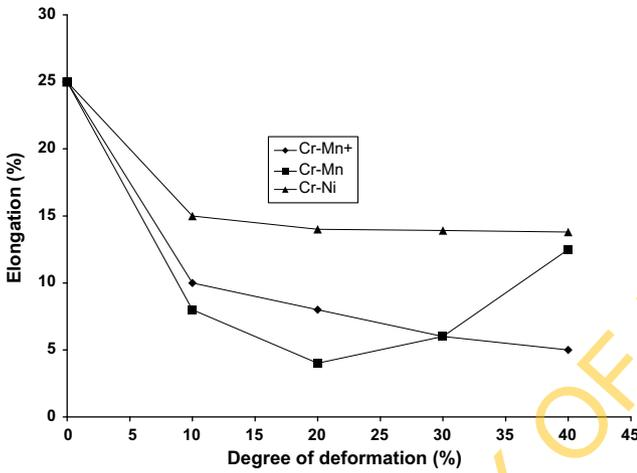
Fig. 2b. Variation of elongation with degree of deformation at 350 °C.
