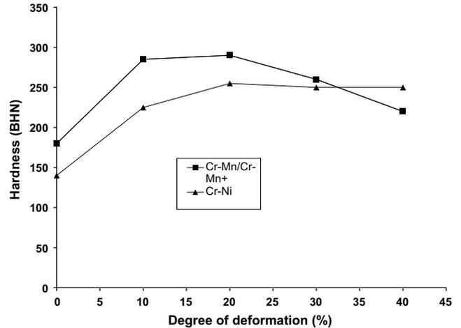
Fig. 5c. Variation of hardness with degree of deformation at 650 °C.
