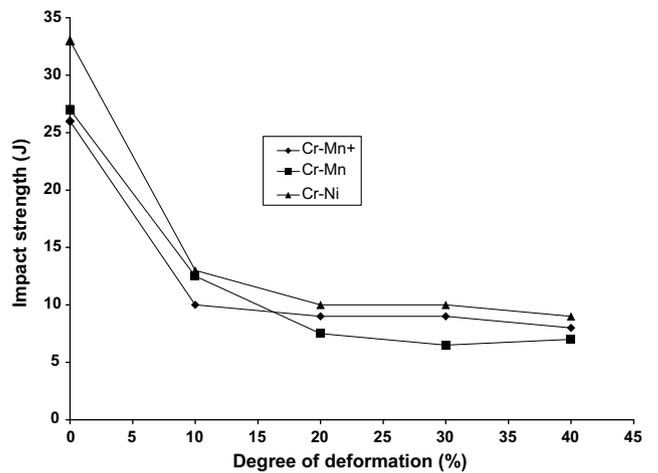
Fig. 3c. Variation of impact strength with degree of deformation at 650 °C.
