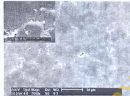
Figure 11: Simulated HAZ microstructure in a sample heated to 1225°C for 1s and water quenched.
