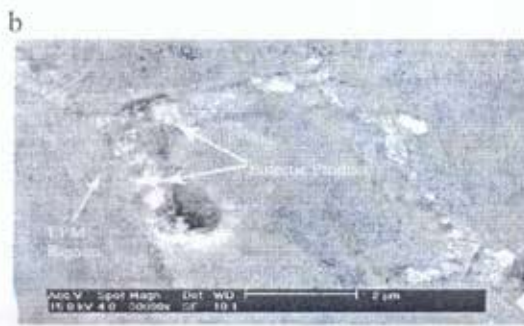
Figure 13: SEM micrographs showing the extent of (a) liquid film migration at low magnification in thermally simulated microstructure with applied 10% external compressive strain, (b&c) higher magnification of some marked regions from 'a' intergranular liquid film migration.
