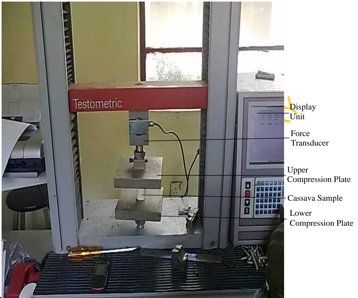
Plate 3.5: Universal Testing Machine used for Compressive Strength Tests
