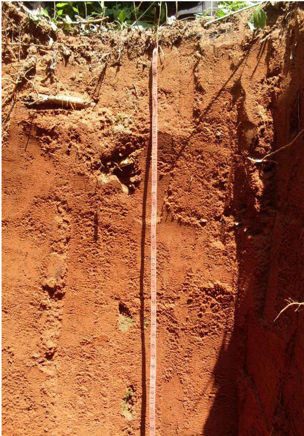
Plate 4.3: Soil profile of Orlu Series ( Rhodic Haplaudult or Acric Nitisol (Dystric) at Block MN1, Iyanomo
