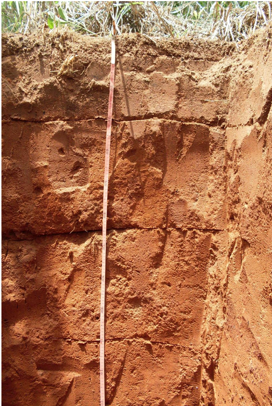
Plate 4.1: The soil profile of Alagba series [Rhodic Haplaudult or Lixic Nitisol (Eutric)] at Iyanomo.
