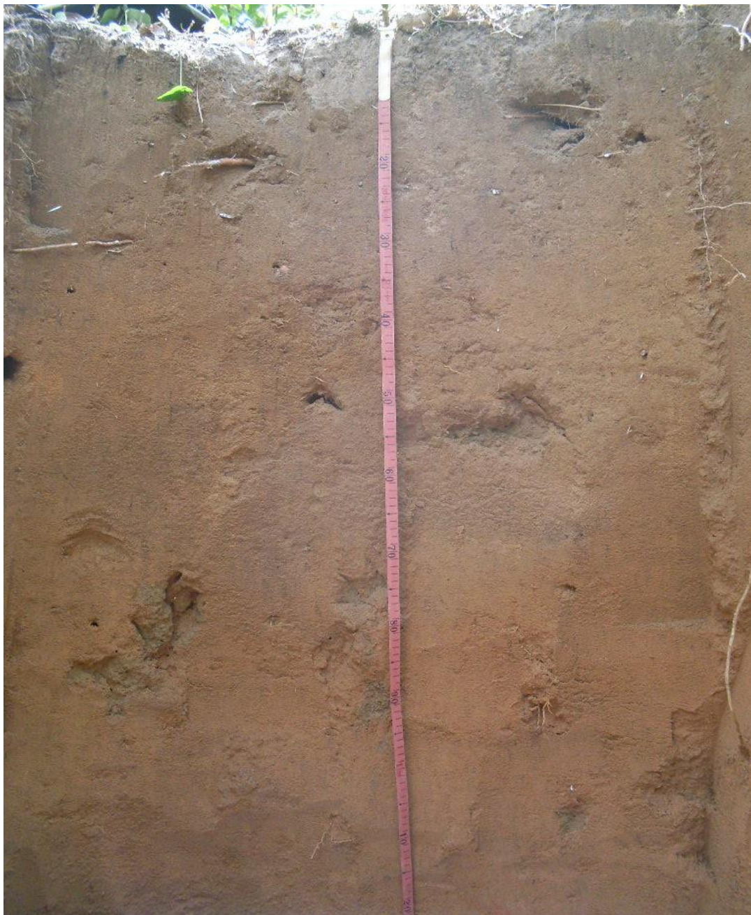
Plate 4.1: Profile of Ahiara Series [Typic Dystrudept or Haplic cambisol (Eutric)] Block K12, Iyanomo
