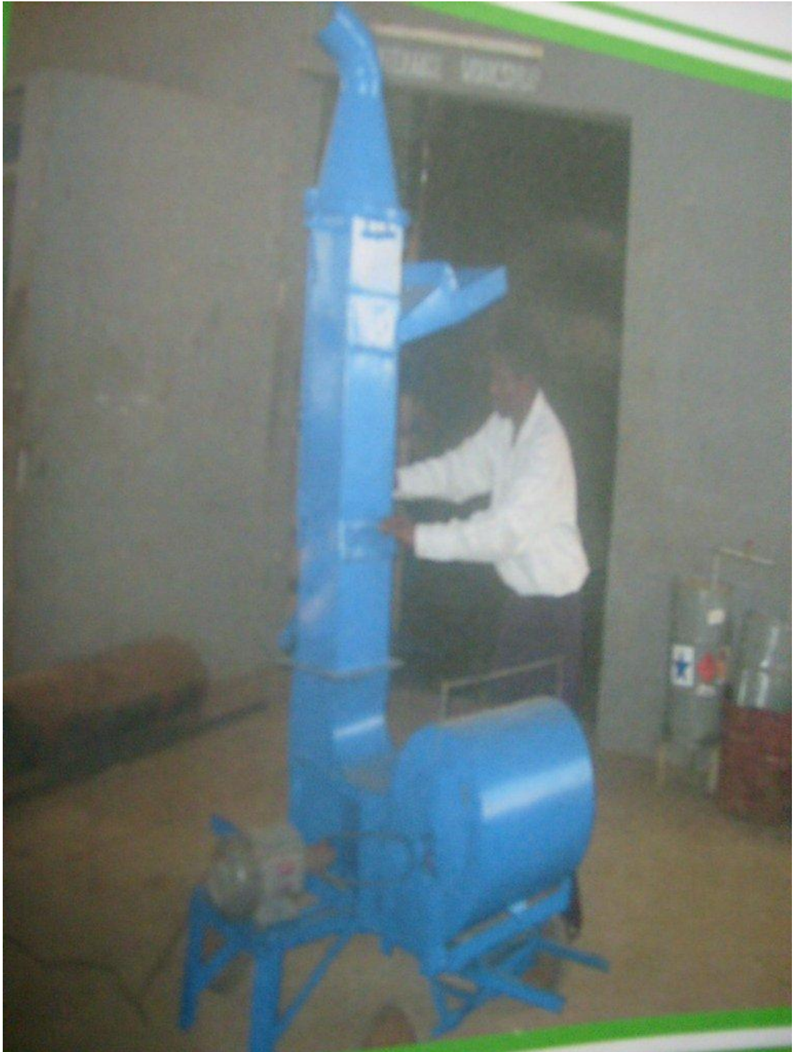
Plate A2. A pneumatic separator for cowpea at college of Agriculture I. A. R. &T, Ibadan
