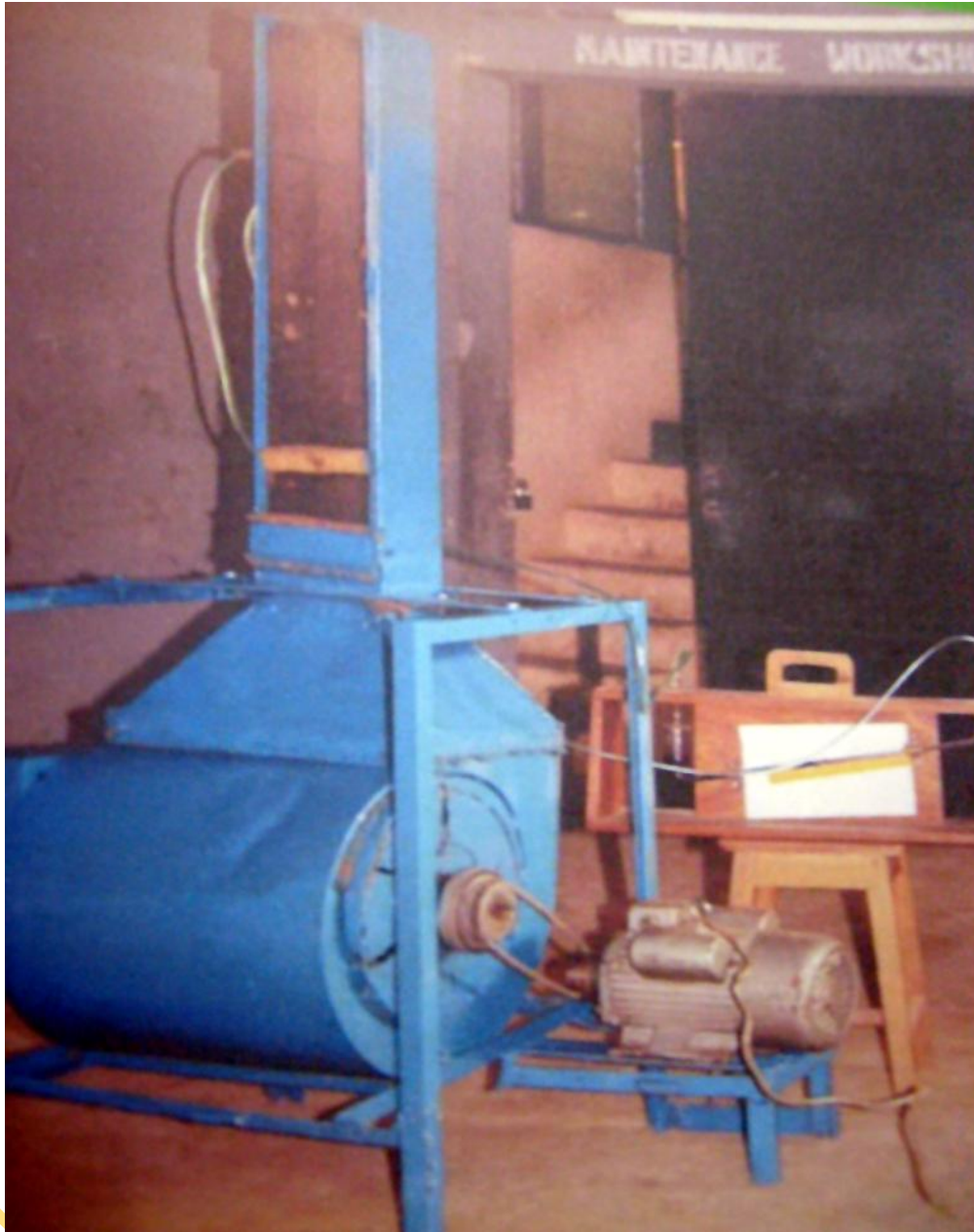
Plate A3. A vertical wind tunnel used for measuring the terminal velocity of particles of 7m/s and above
