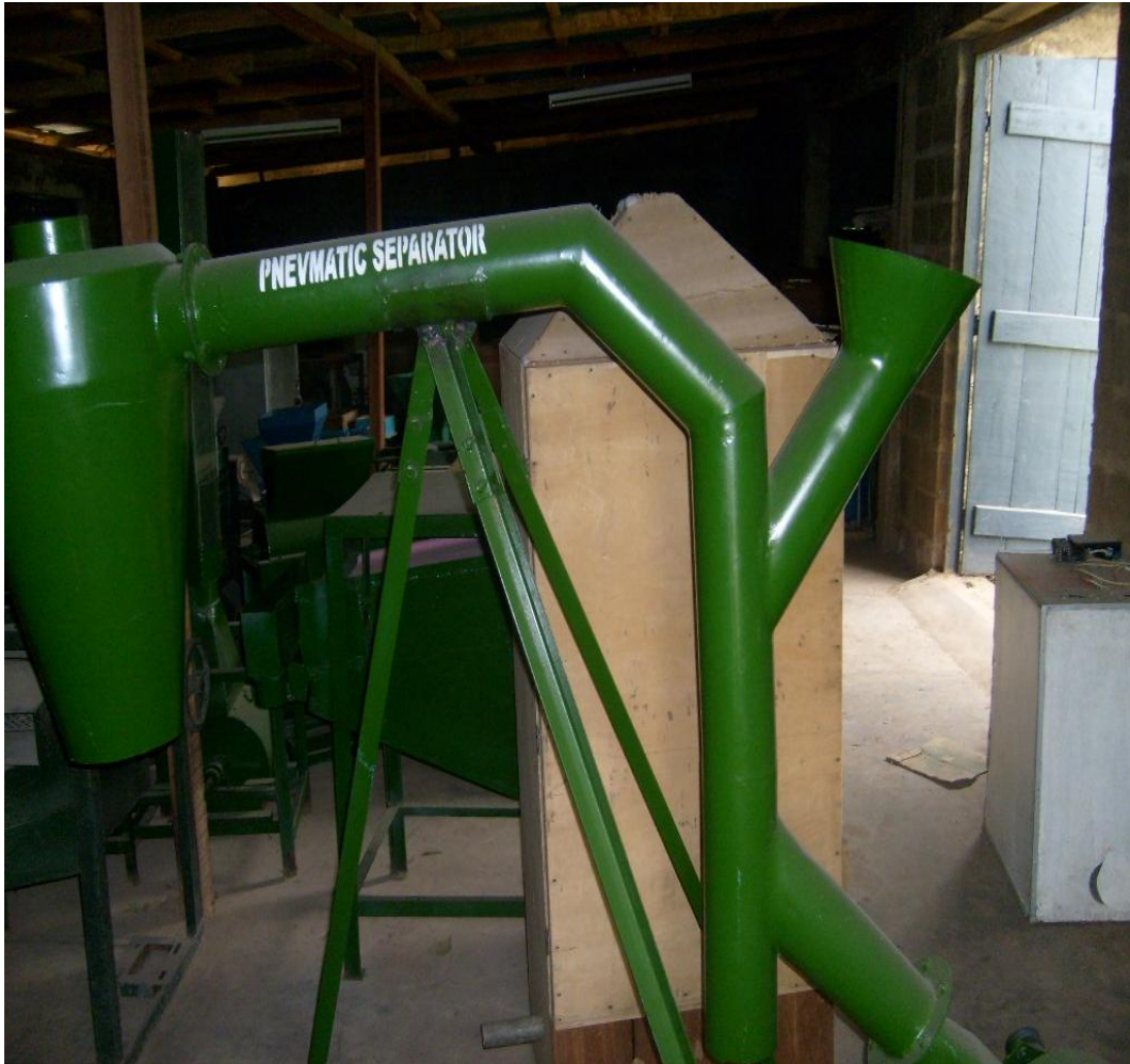
Plate A1. A pneumatic cleaner at the department of Agricultural and Environmental Engineering, University of Ibadan
