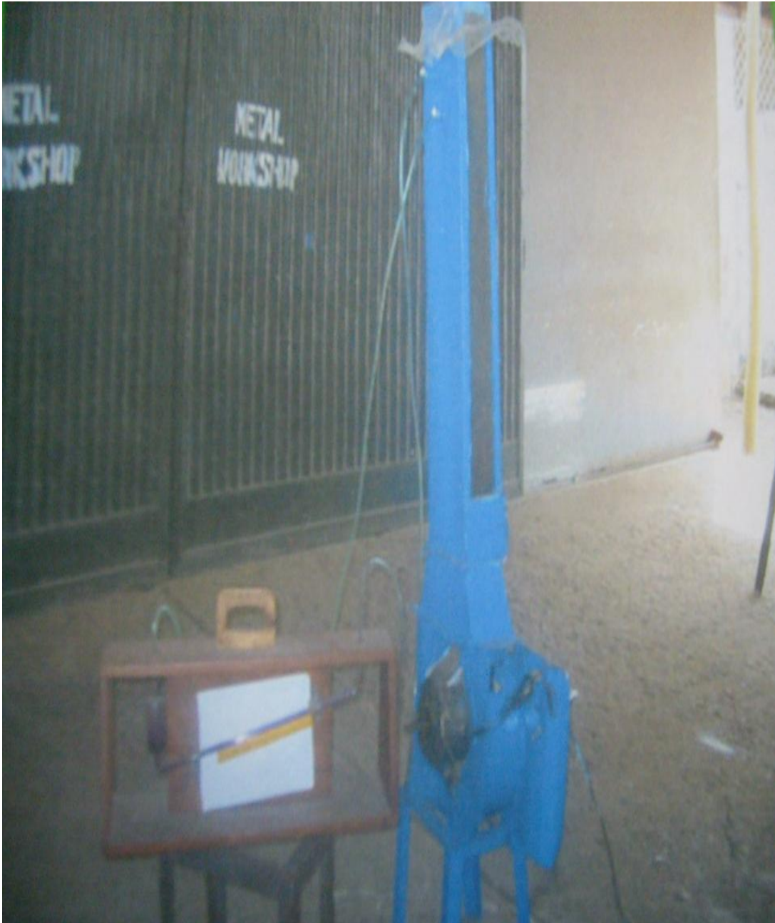
Plate A4. A vertical wind tunnel for measuring lower values of terminal velocities
