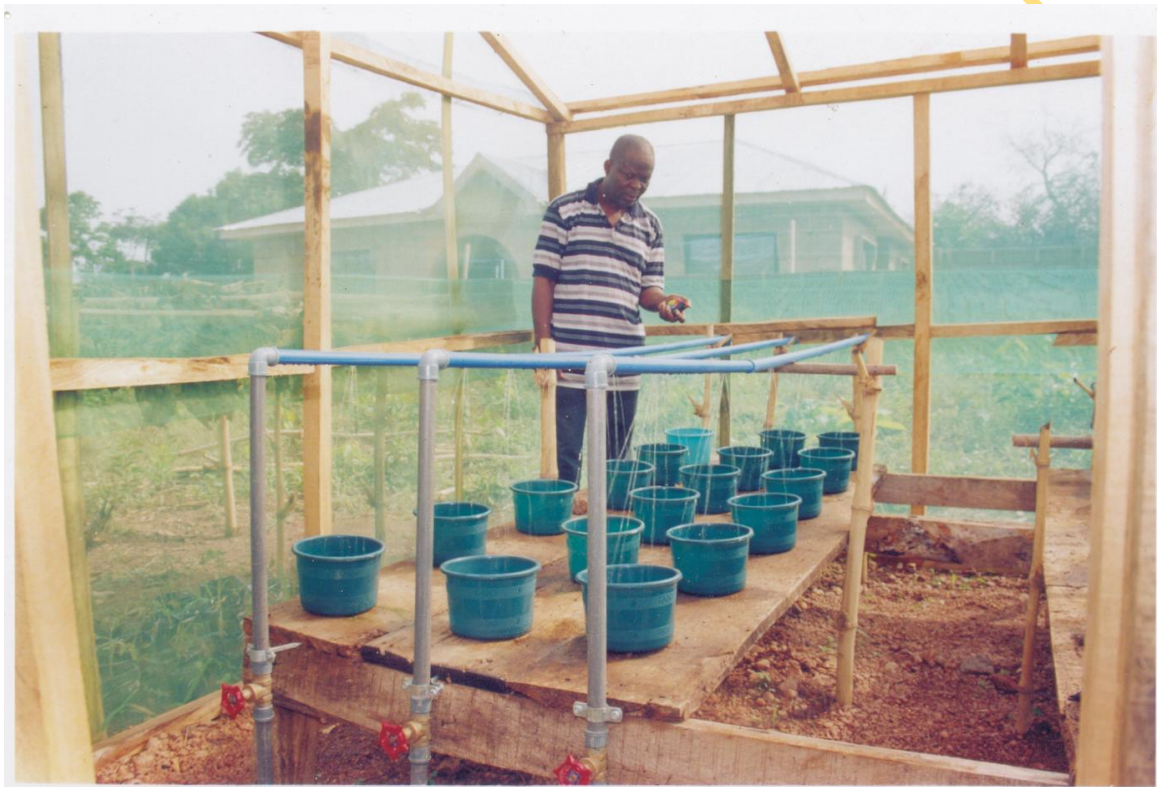
Plate 8: Experiment to determine the discharge of the sprinkler
