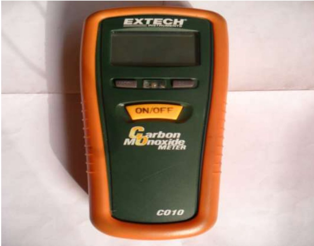
Plate 3.8: Extech carbon monoxide monitor model CO10
