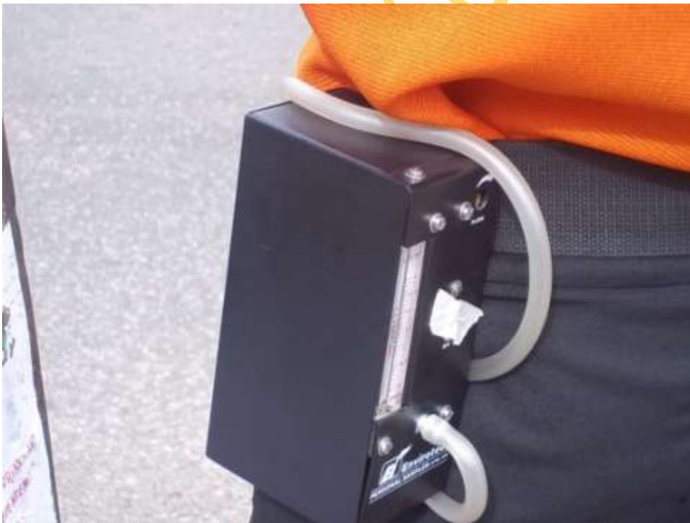
Plate 3.5: Sampler unit strapped to the belt of a traffic warden
