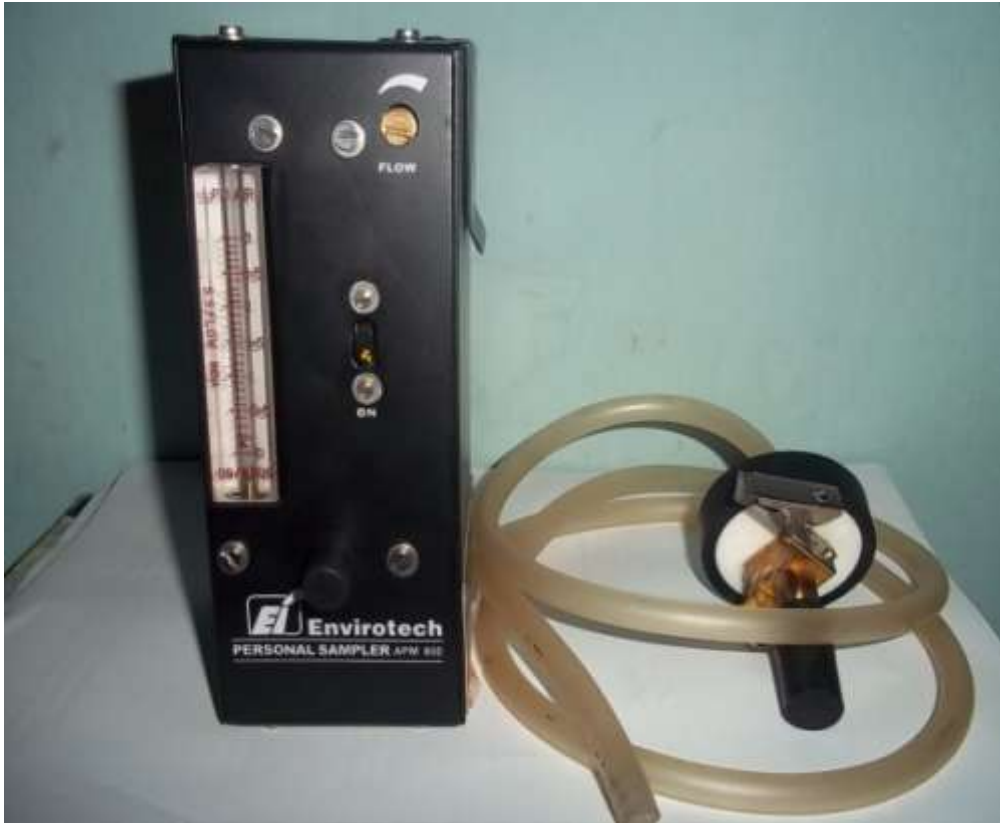
Plate 3.2: Envirotech personal respirable dust sampler model APM801
