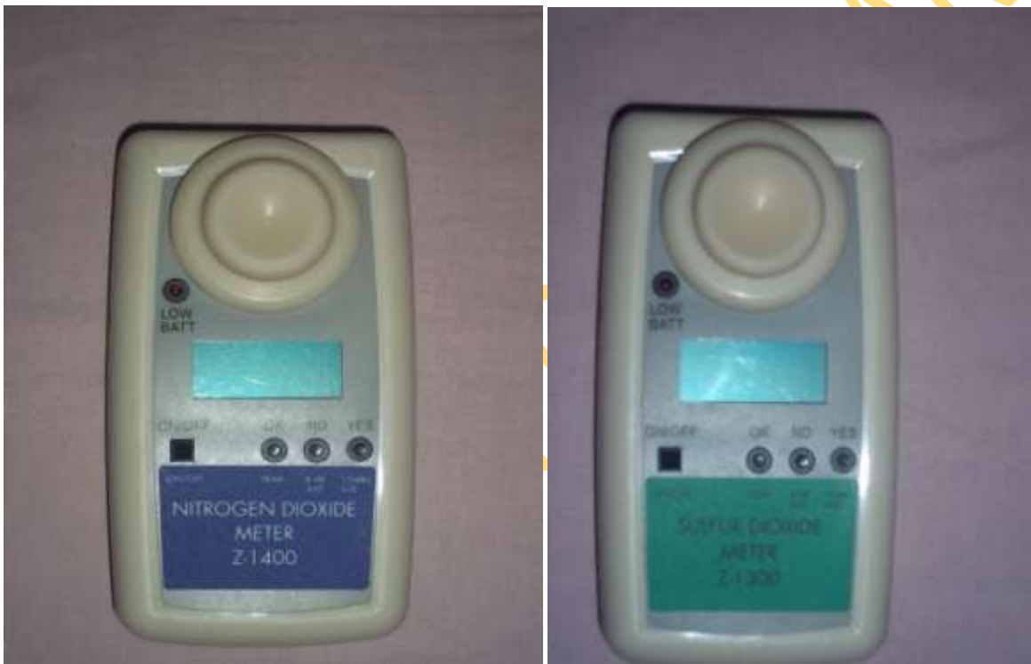
Plate 3.7: Air Samplers: nitrogen dioxide and sulphur dioxide monitors model Z-1400 and Z-1300 respectively.
