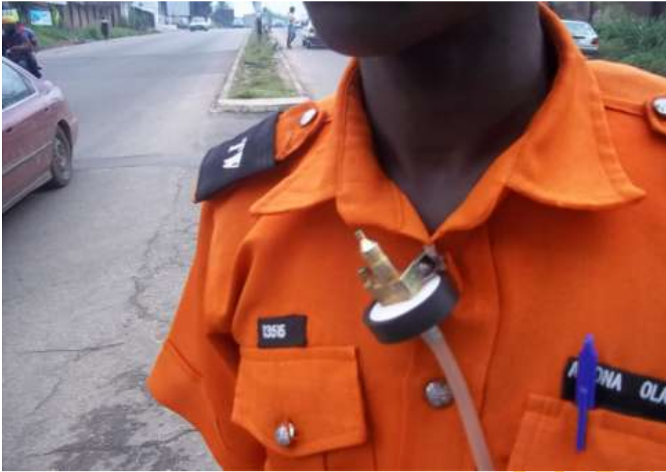
Plate 3.4: Shows the sampling head attached to the shirt of a traffic warden
