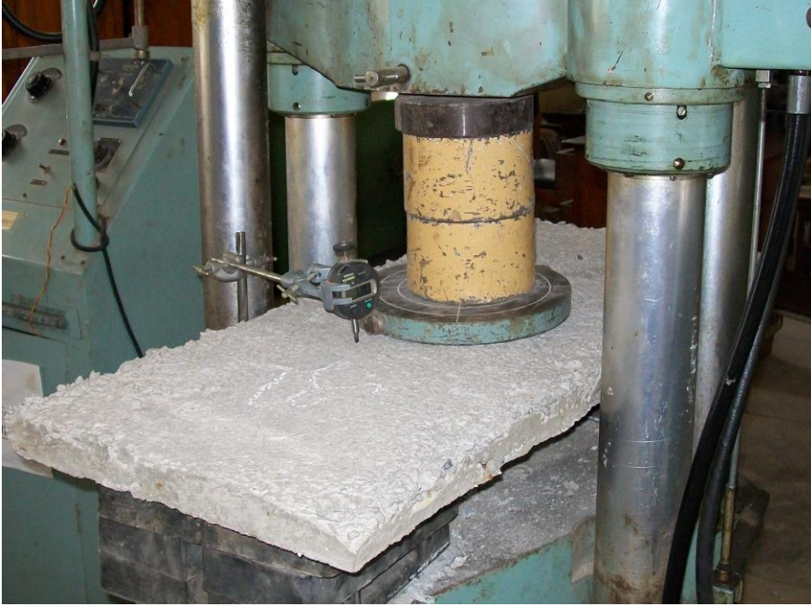
Plate 4: Test arrangement for a slab sample
