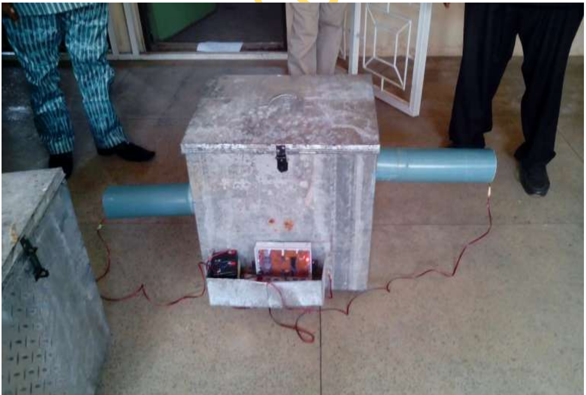
Plate 4.8: Back view of extractor with controller and batteries
