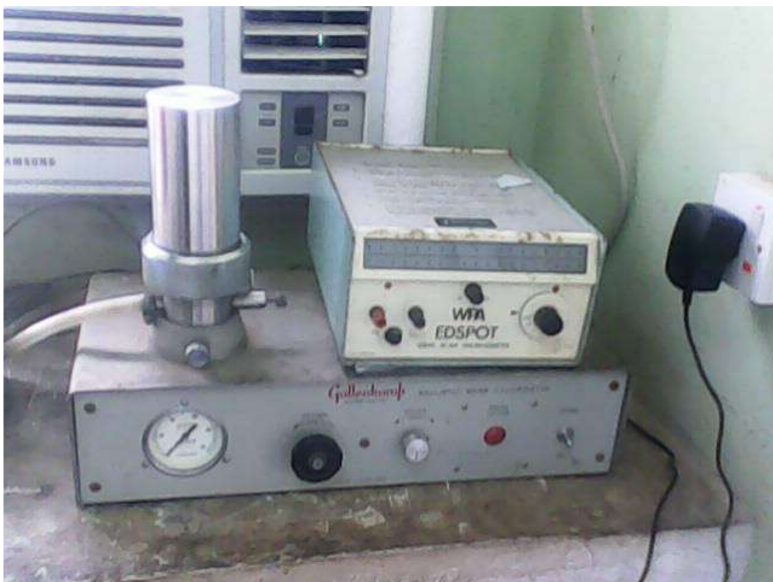
Plate 3.19: Gross energy determination using Gallenkamp Ballistic Bomb Calorimeter
