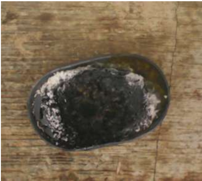
Plate 3.11: Activated carbon produced from sawdust with KOH
