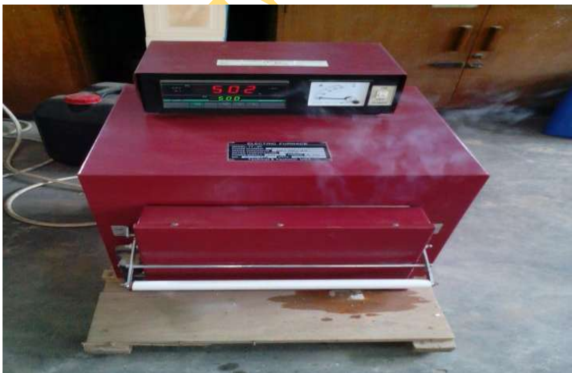
Plate 3.10: Furnace in operation at 500°C for heating the sawdust and KOH
