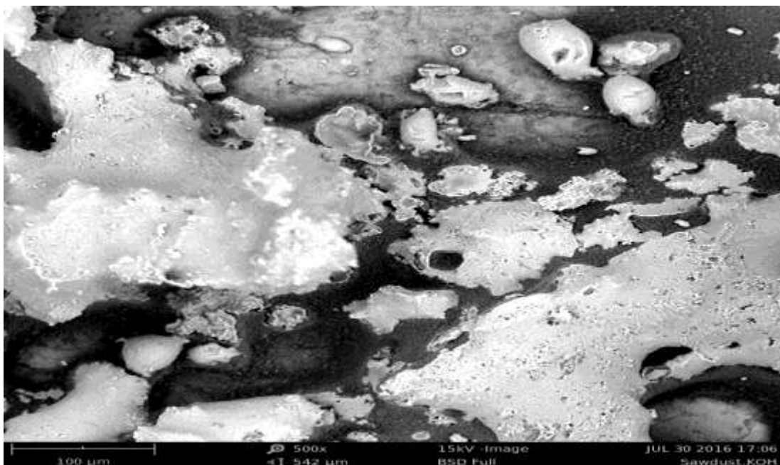
Plate 4.4: SEM Image of activated carbon from sawdust and KOH at 500 times magnification showing the particle size weighted by volume
