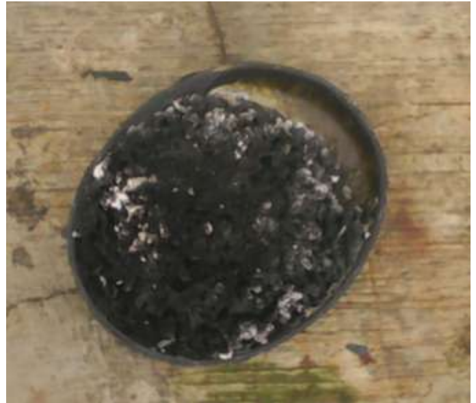
Plate 3.12: Activated carbon produced from sawdust with NaOH
