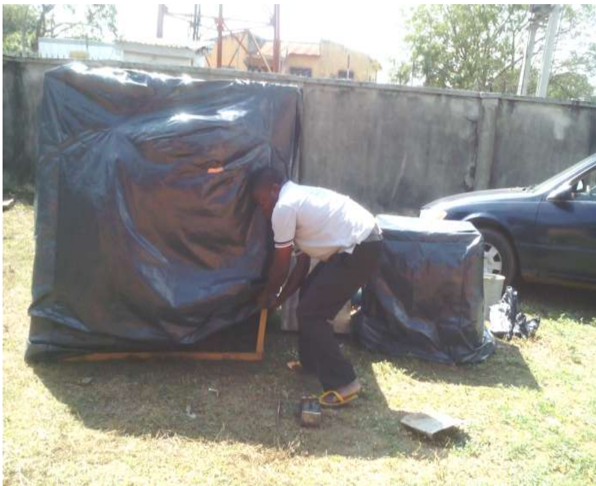
Plate 3.18: Measurement of baseline carbon dioxide
