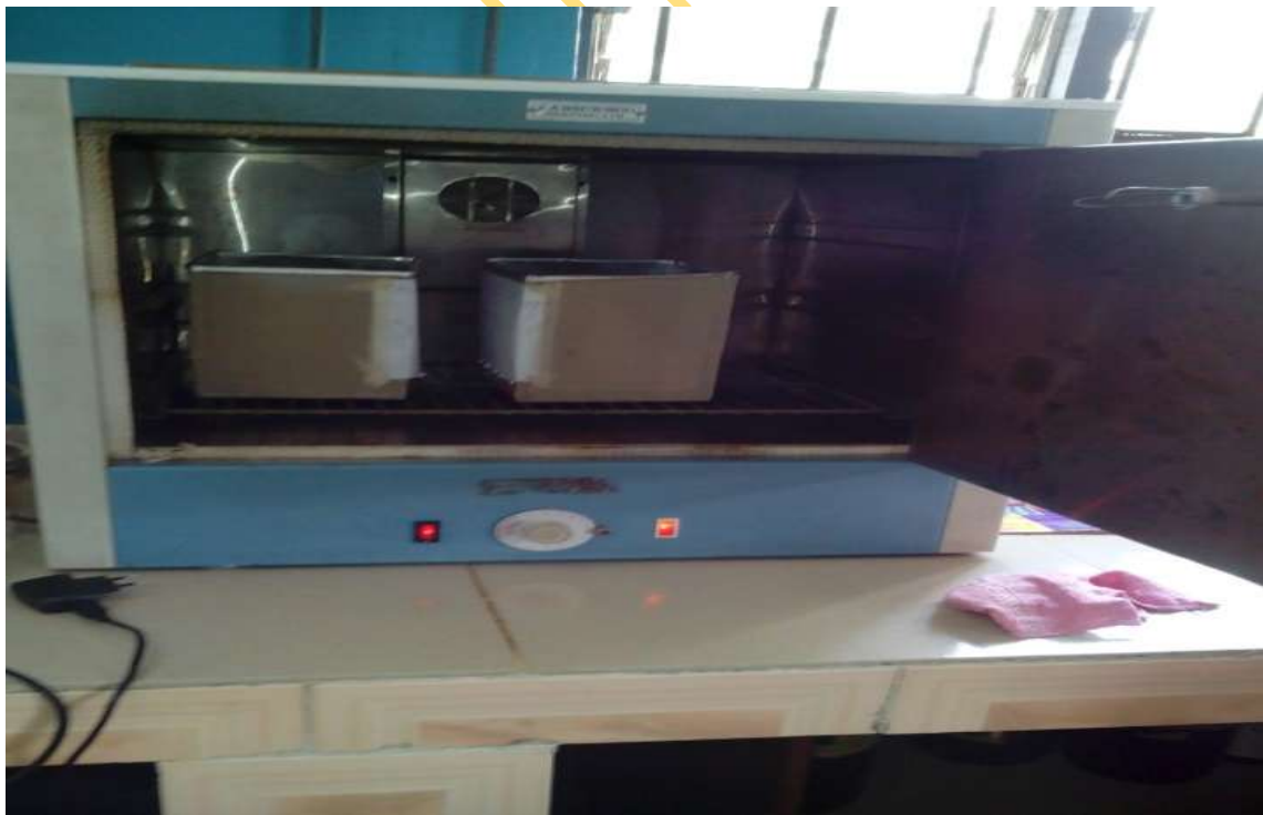
Plate 3.8: Drying of sawdust in an Oven at 110°C for 24 hours
