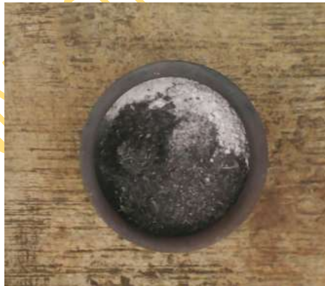
Plate 3.13: Activated carbon produced from sawdust with \text{Ca}(\text{OH})_2
